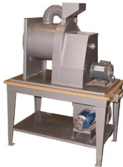
Gambar 19. Alat sortasi mekanis seed cleaner
