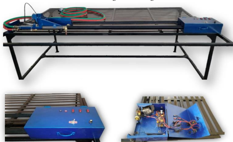
Gambar 3. Hasil perencanaan gas cutting machine
