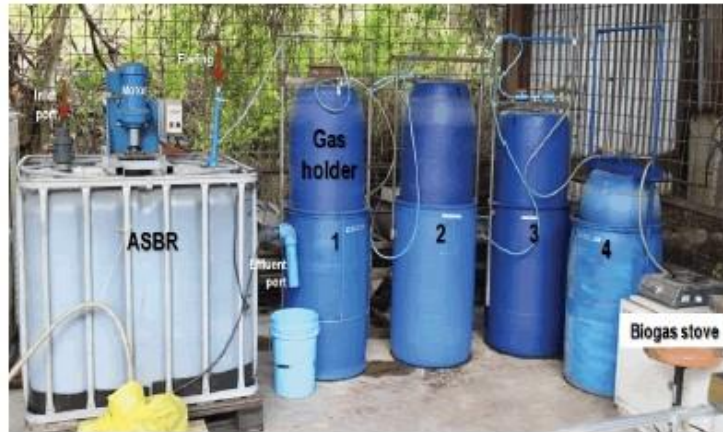
Figure 2. Fabricated ASBR and biogas holders. Capacity: ASBR, 1,000 L; gas holders, 245 L.
