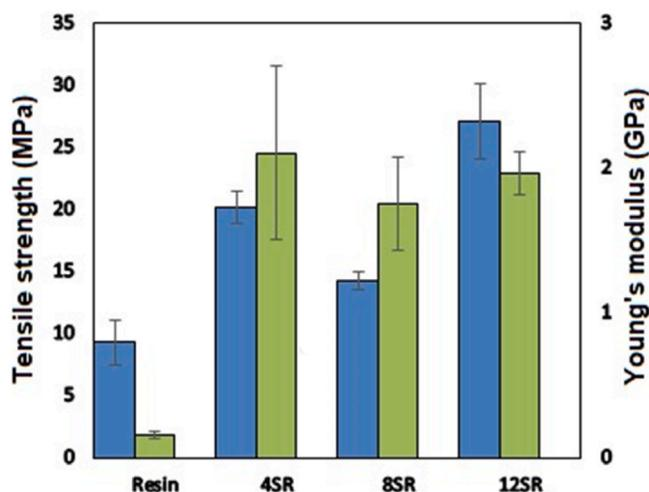
**Fig. 8.** Tensile strength and the Young's modulus of neat epoxy adhesive resin, and composites based on cellulose fibers fabricated from oil palm empty fruit bunch fibers subjected to 4, 8, and 12 pretreatment cycles with a 4 wt% aqueous solution of NaOH followed by blending (4SR, 8SR, and 12SR, respectively).
