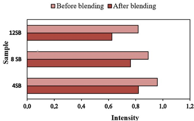
Fig. 6. The intensities of Fourier-transform infrared spectra peaks of lignin (1639 cm<sup>-1</sup>) comparison between before and after blending in different pretreatments.
