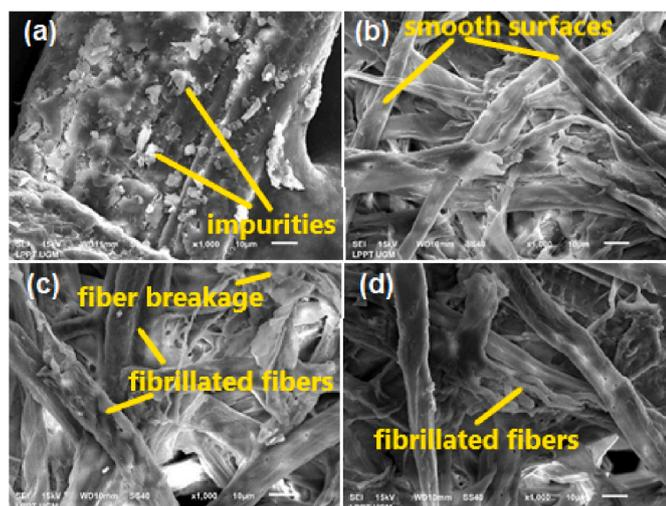
Fig. 2. SEM images of (a) raw OPEFB fibers and cellulose fibers fabricated from OPEFB fibers subjected to (b) 4, (c) 8, and (d) 12 pretreatment cycles with a 4 wt% aqueous solution of NaOH followed by blending.
